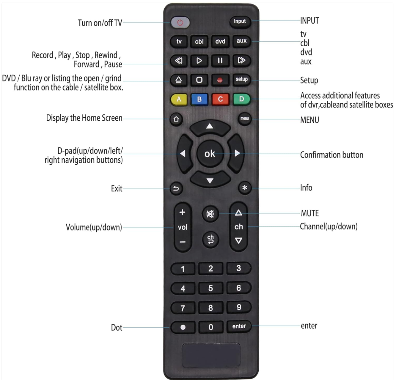
Image 4: Detailed diagram of the NJALNKHM G009 remote control, with labels indicating the function of each button for easy identification and use.
