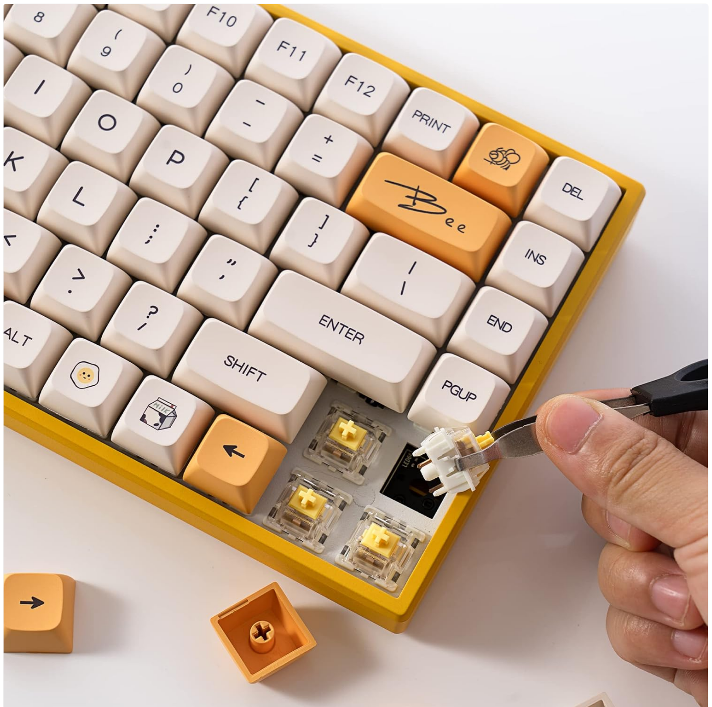
Image: A hand using a switch puller to remove a Gateron Yellow switch from the BOYI KD84 keyboard, demonstrating the hot-swappable feature.
