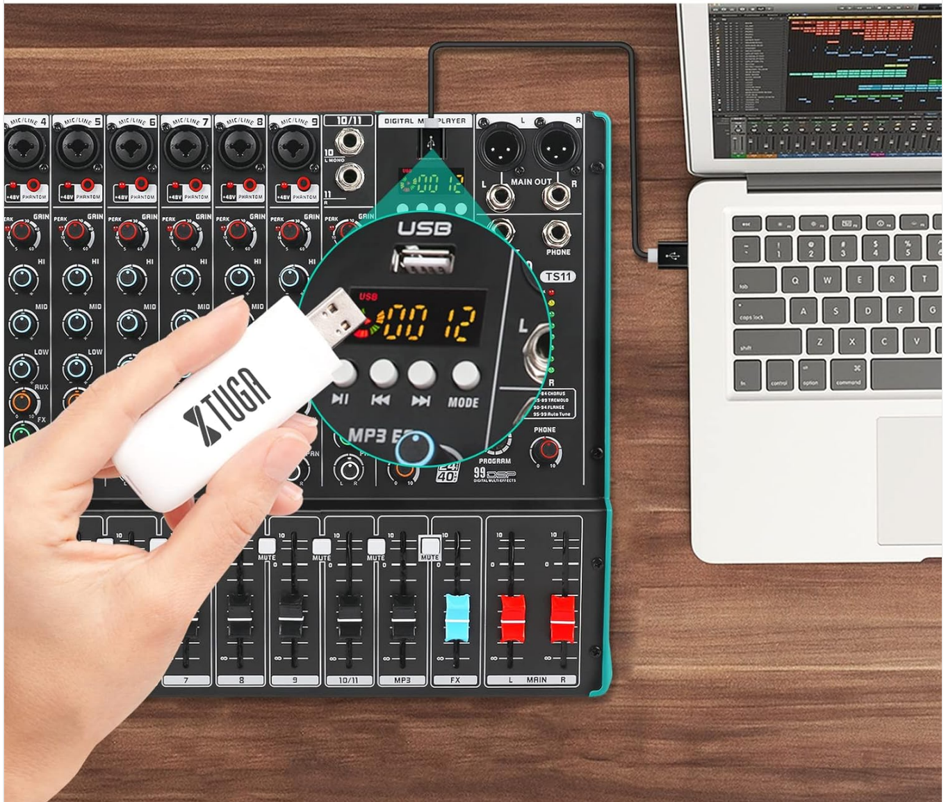
Figure 7: The USB interface, demonstrating how to connect a USB flash drive for MP3 playback or a computer for recording and playback.
