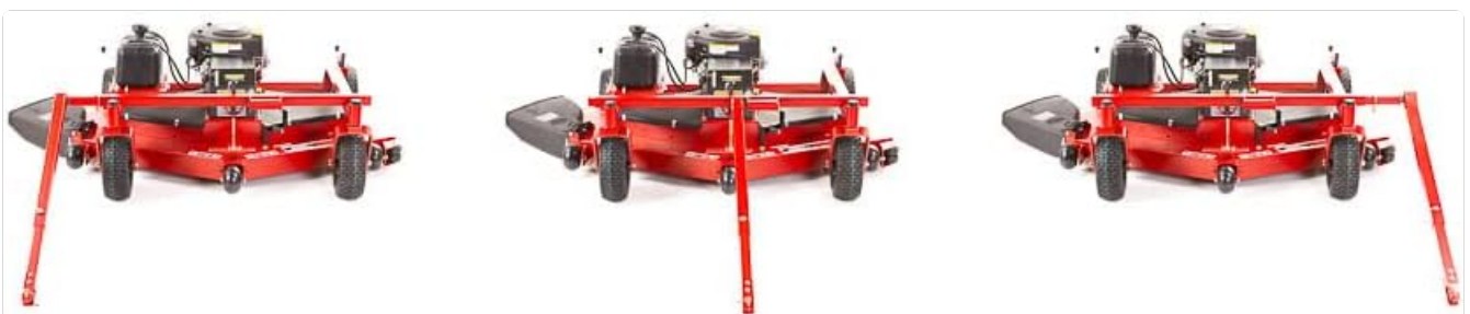
Figure 4.2: The adjustable hitch allows for offset towing positions.
