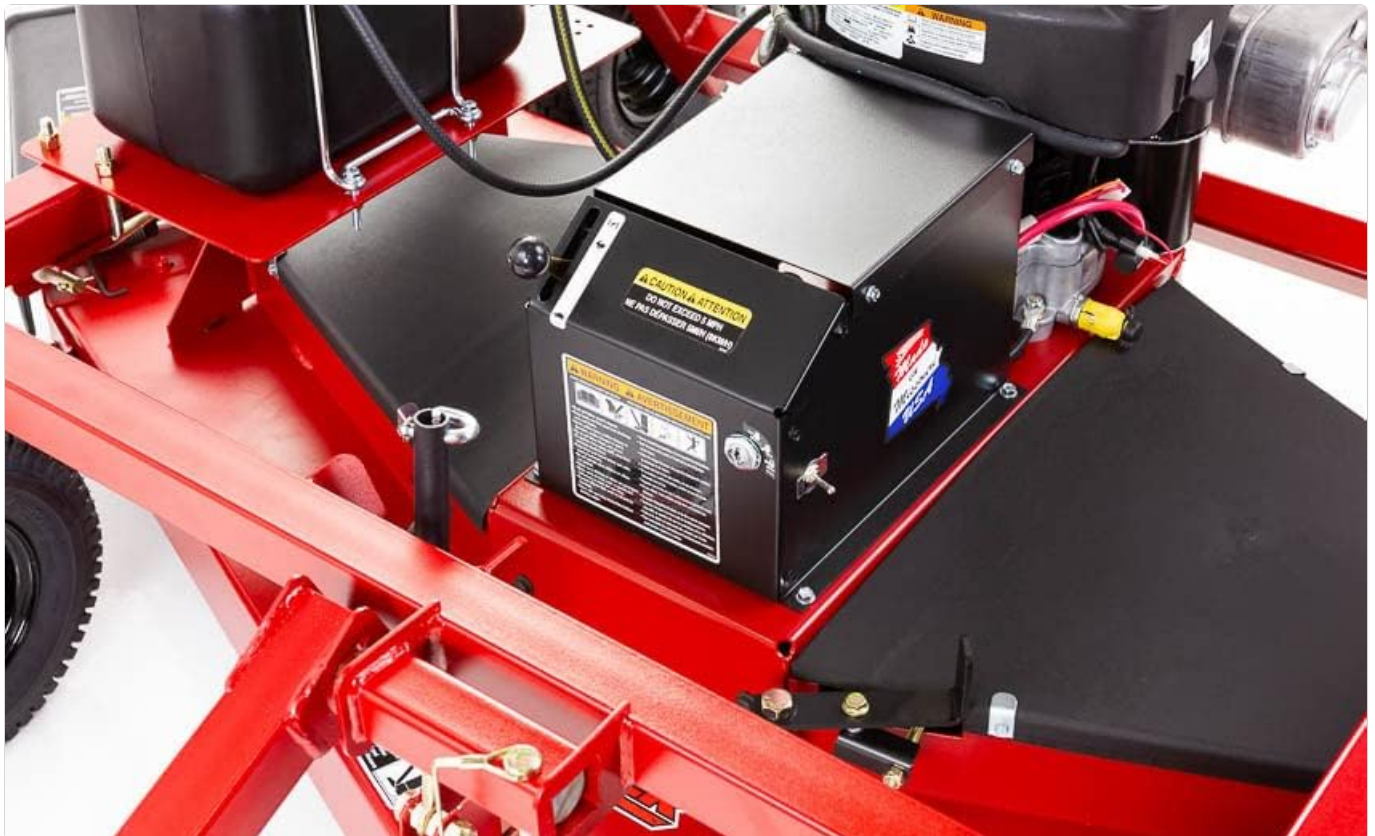
Figure 4.1: Cutting height adjustment lever. Adjusting this lever raises or lowers the mower deck.
