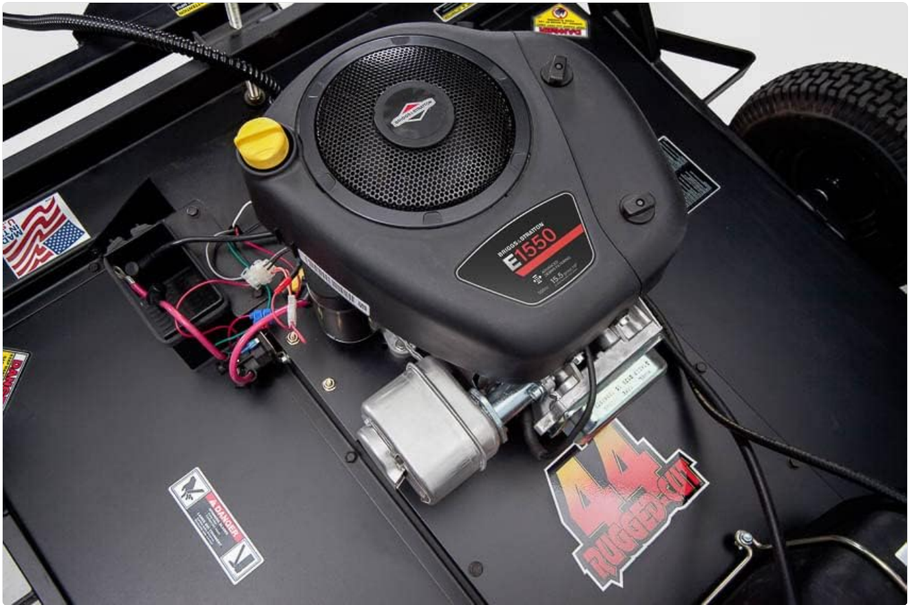
Figure 3.4: The powerful Briggs & Stratton 15.5 HP engine drives the cutting blades.
