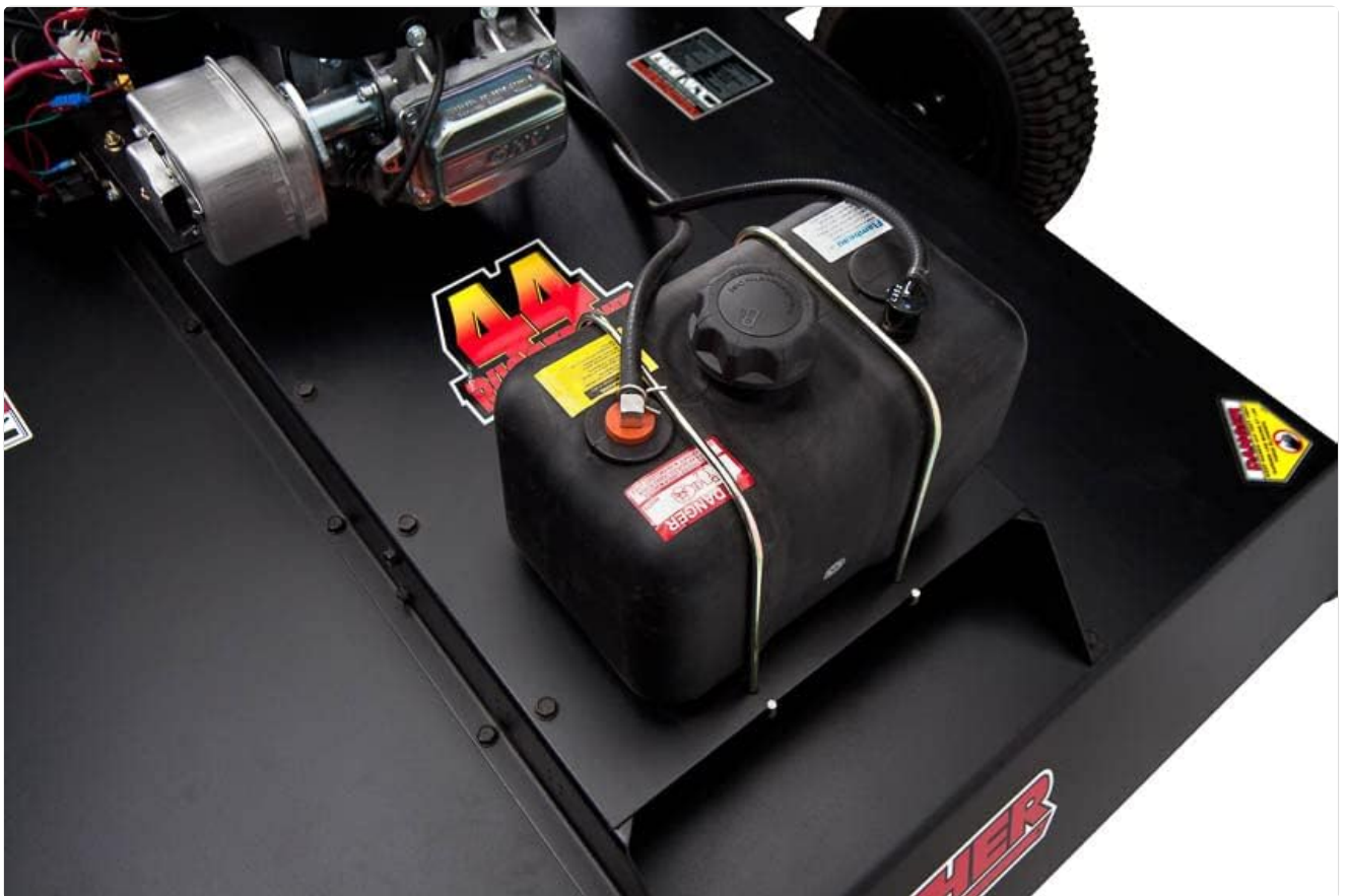
Figure 3.3: The 2.5-gallon fuel tank ensures extended run time.
