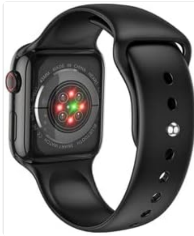
Image: Rear view of the BOROFONE BD1 Smart Watch, highlighting the heart rate sensors and magnetic charging contacts.
