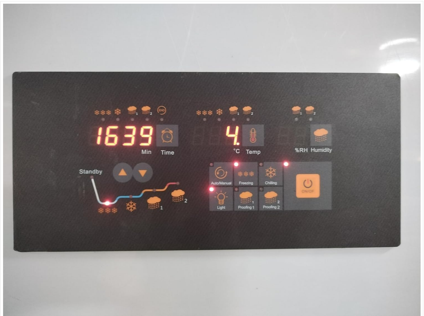
Image 4.1: Close-up of the touch control panel with temperature, humidity, and function settings.
