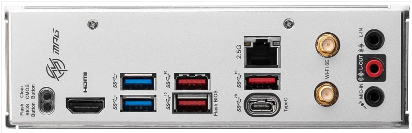
Figure 4: Rear Input/Output (I/O) panel detailing available ports and connectors.
