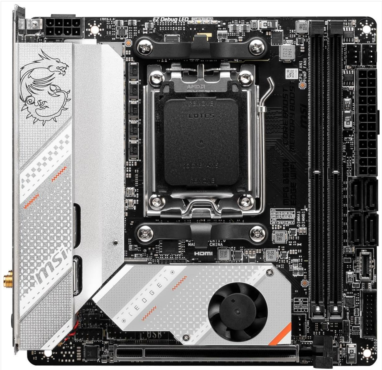
Figure 3: Top-down view of the motherboard layout, highlighting the CPU socket, DDR5 memory slots, and M.2 Shield Frozr.
