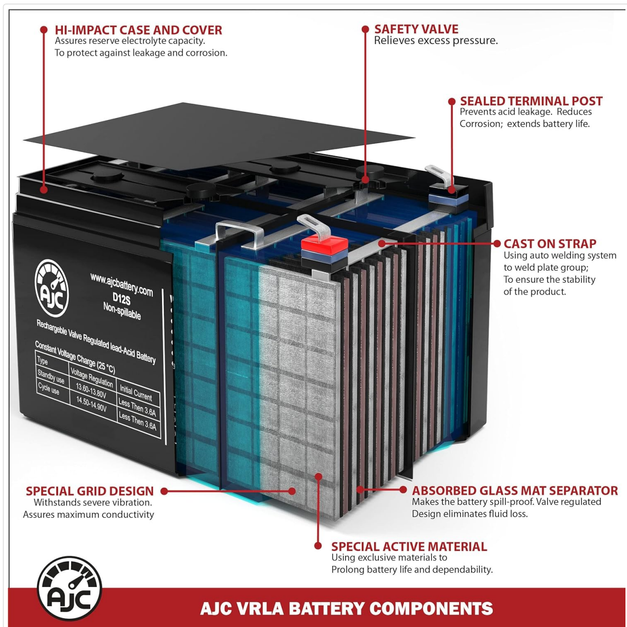
Figure 3.1: Internal components of an AJC VRLA battery, highlighting features such as the hi-impact case, safety valve, and absorbed glass mat separator for enhanced performance and safety.
