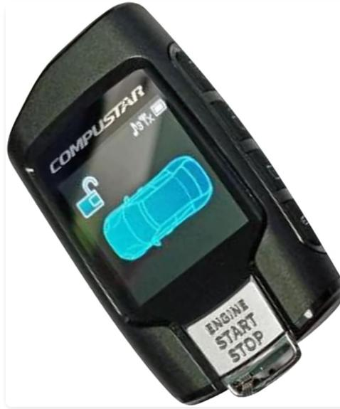
**Image Description:** The Compustar 2WQ9R-FM remote's LCD screen showing the 'Disarm Unlock' status, indicating the vehicle's security system is disarmed and doors are unlocked.
