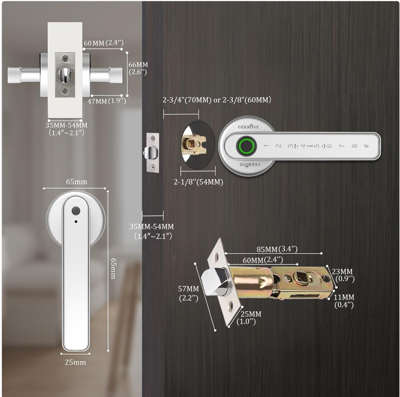
Image: Detailed diagram illustrating the compatible door dimensions and lock buckle measurements for installation.
