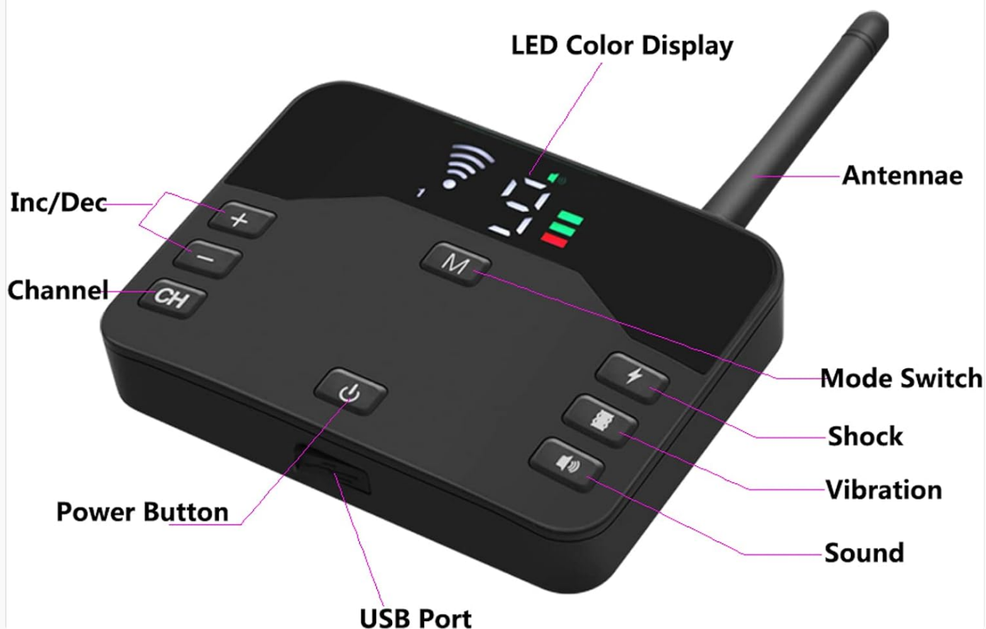
Figure 4.1: Layout of the Transmitter Unit Functions. This diagram labels the LED Color Display, Antennae, Increment/Decrement buttons (+/-), Channel (CH) button, Power Button, USB Port, Mode Switch, Shock button, Vibration button, and Sound button.
