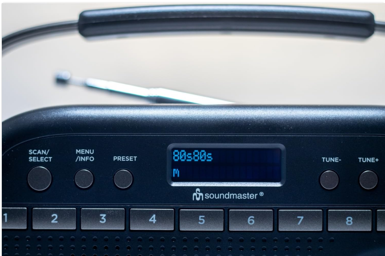
Image 5.1: Top view of the radio showing the display, SCAN/SELECT, MENU/INFO, PRESET buttons, and preset buttons 1-8.
