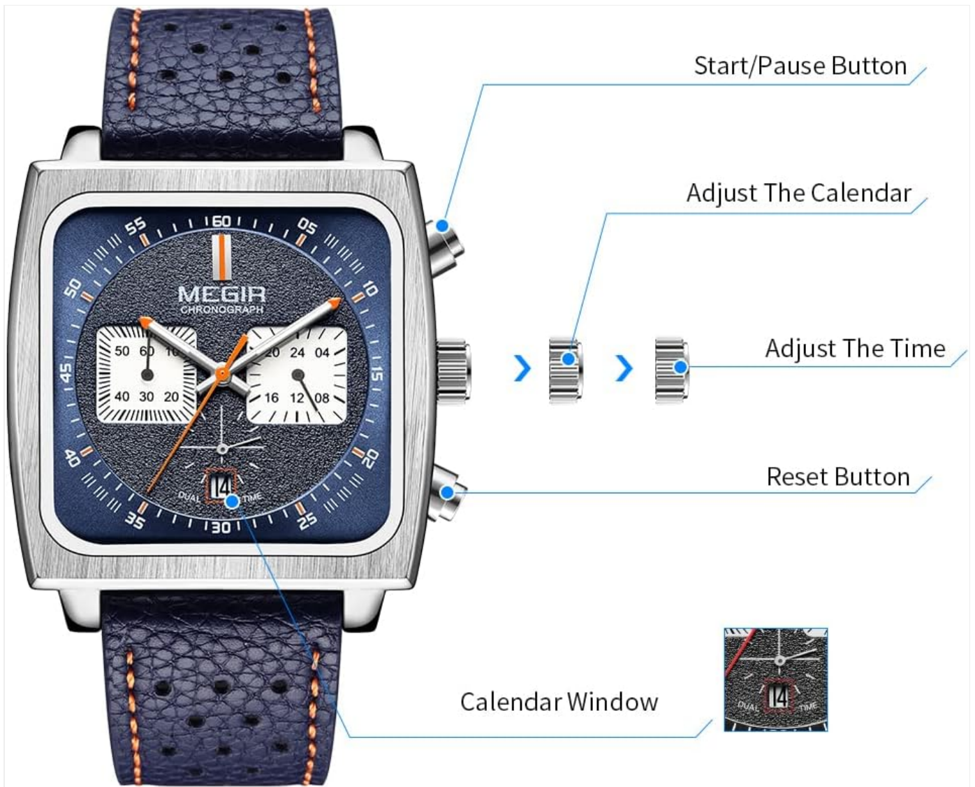
Image 3.1: Watch components and their functions.
