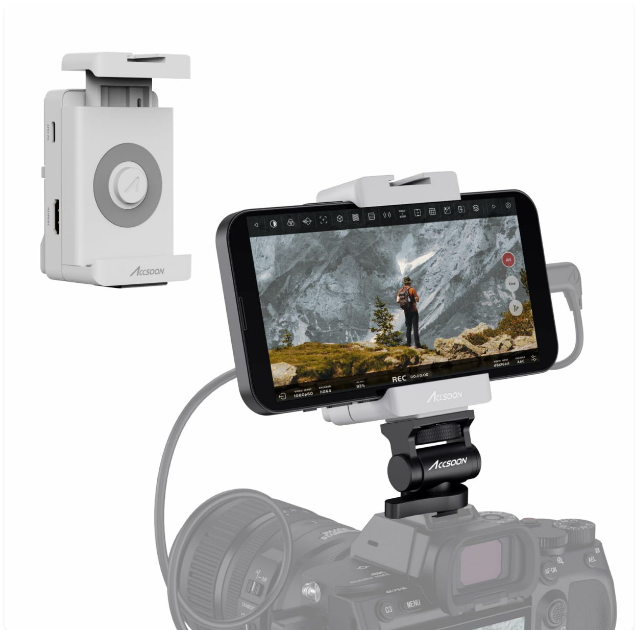
Image 1.1: Accsoon SeeMo adapter connected to a camera, with an iPhone mounted for monitoring.
