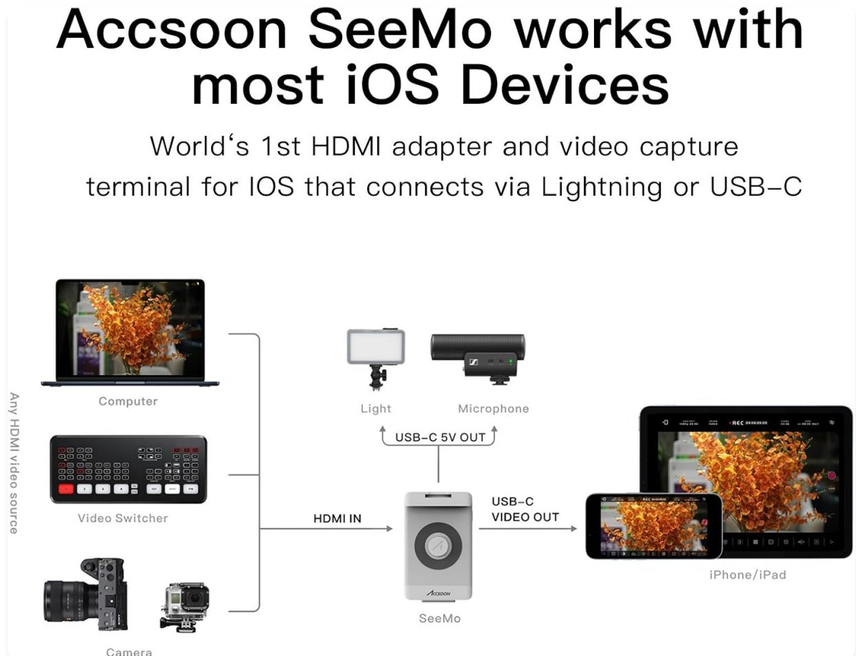
Image 3.2: Connection diagram for Accsoon SeeMo with various devices.
