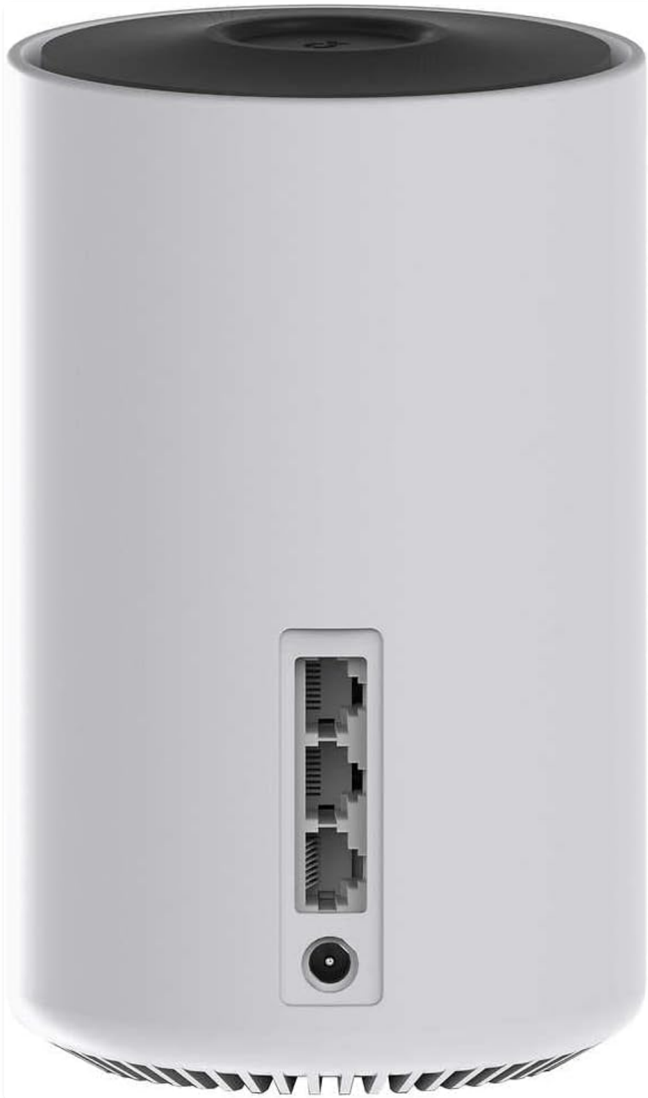
Image: The rear of a Deco AXE5300 unit, highlighting its Ethernet ports and power input.
