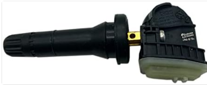
Figure 4: Another view of the LadyCent TPMS sensor, emphasizing its robust construction.
