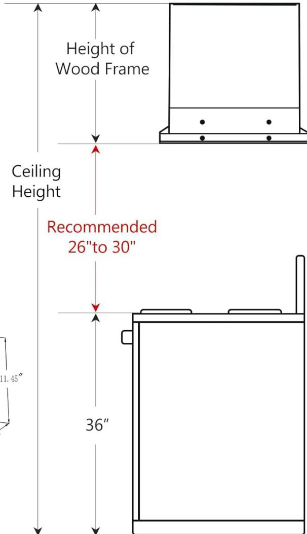
This technical drawing provides precise measurements for the range hood, including installation cut-out dimensions and recommended ceiling height, crucial for proper fitting and setup.
