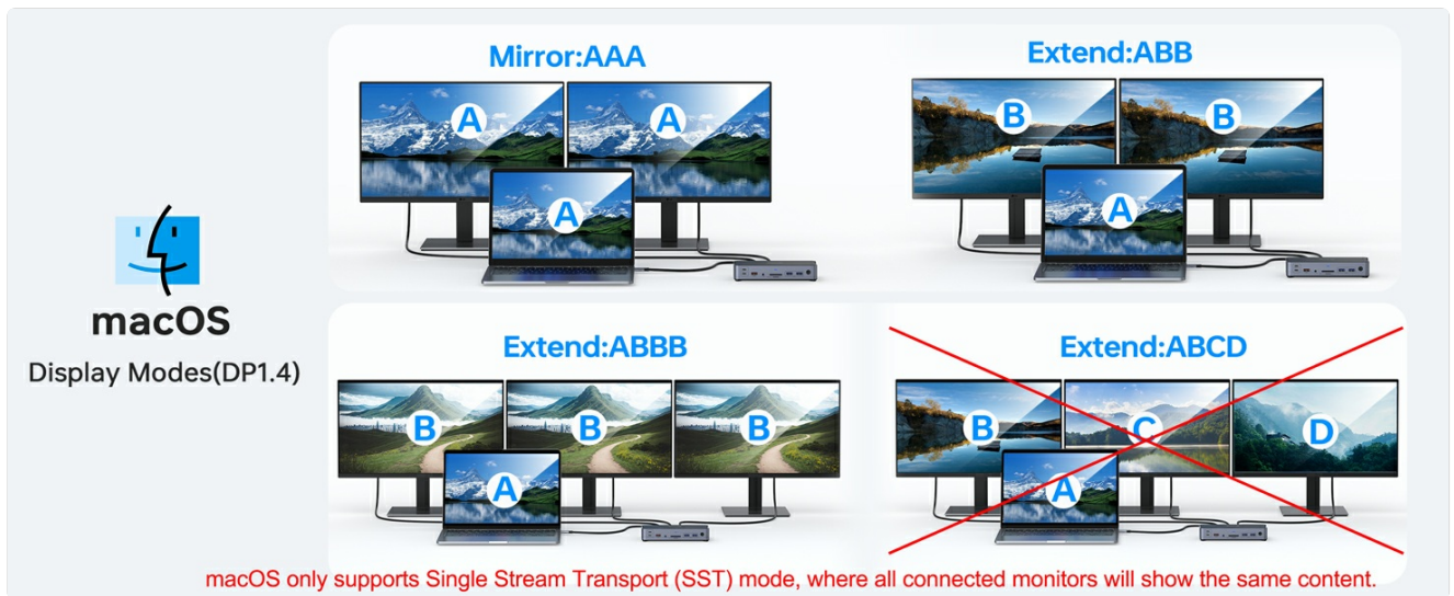
Figure 6: macOS display configurations, highlighting the SST mode limitation for extended displays.
