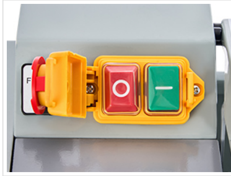
Figure 2: Emergency stop button for immediate machine shutdown.
