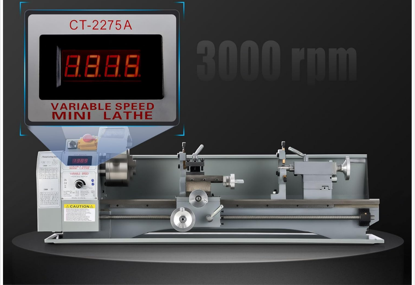
Figure 7: Digital display for monitoring spindle speed and continuous control knob.
