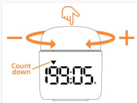
Image 3: Diagram showing how to rotate the timer's top to set the countdown time.
