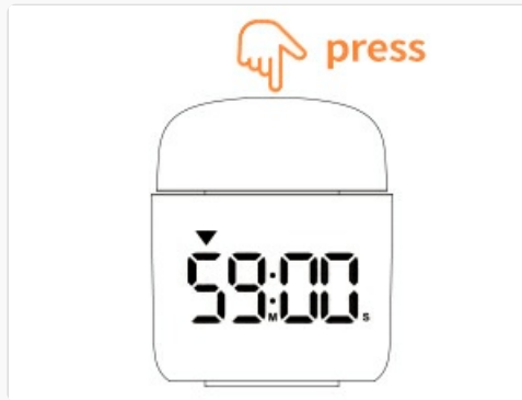
Image 5: Diagram showing a finger pressing the top button to start or pause the timer.
