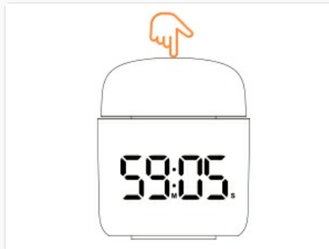
Image 6: Diagram showing a finger pressing and holding the top button to reset the timer to zero.
