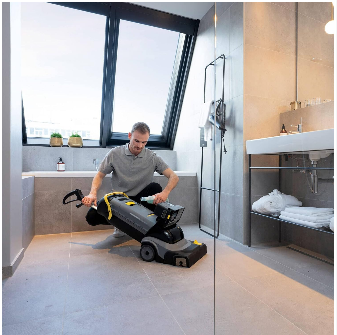
Figure 5: A wider shot of a person filling the fresh water tank of the Kärcher BR 30/4 C BP in a bathroom setting. This provides context for the machine's use and the ease of access to the tank.
