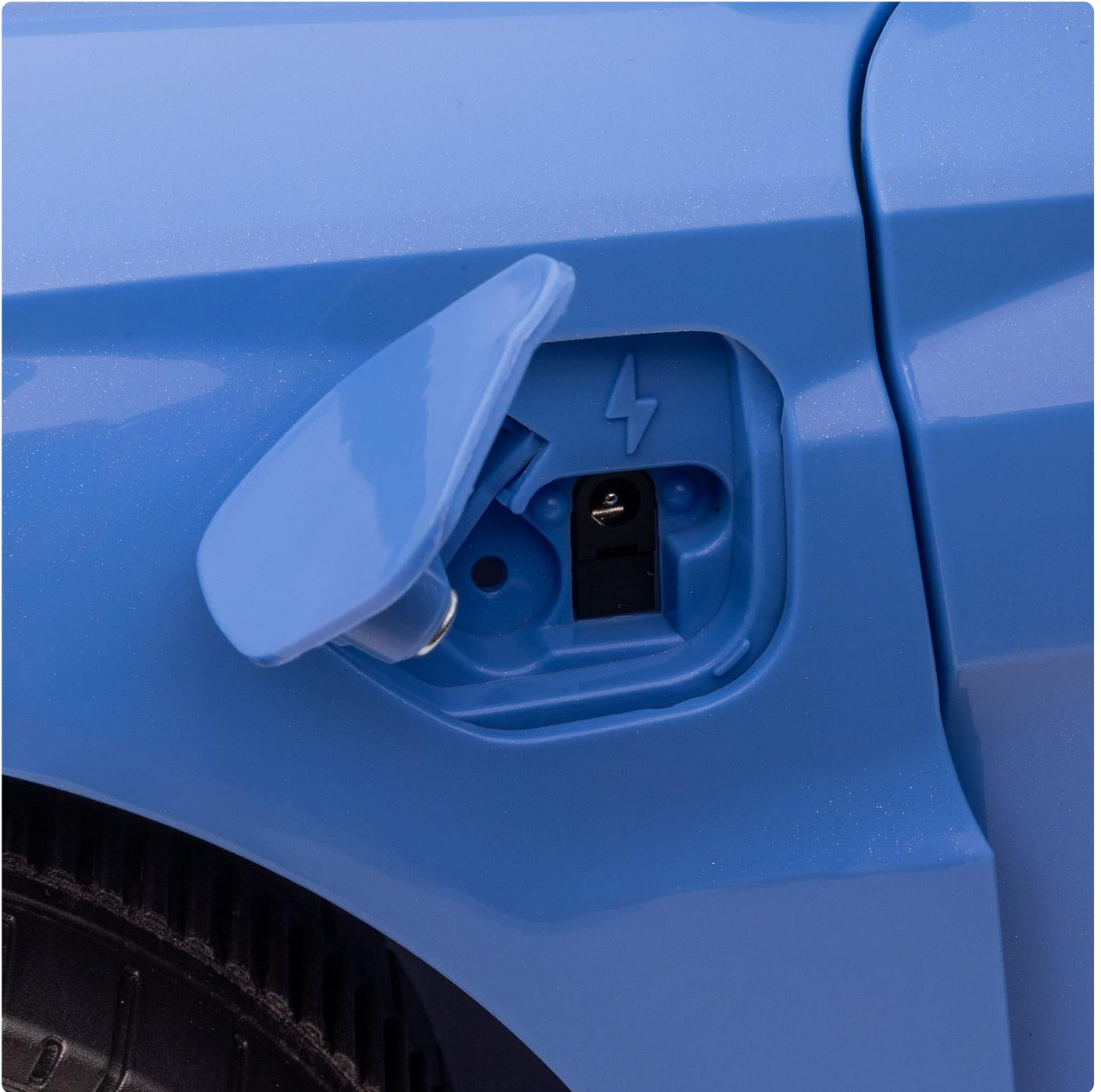
Figure 3: Location of the charging port on the vehicle.
