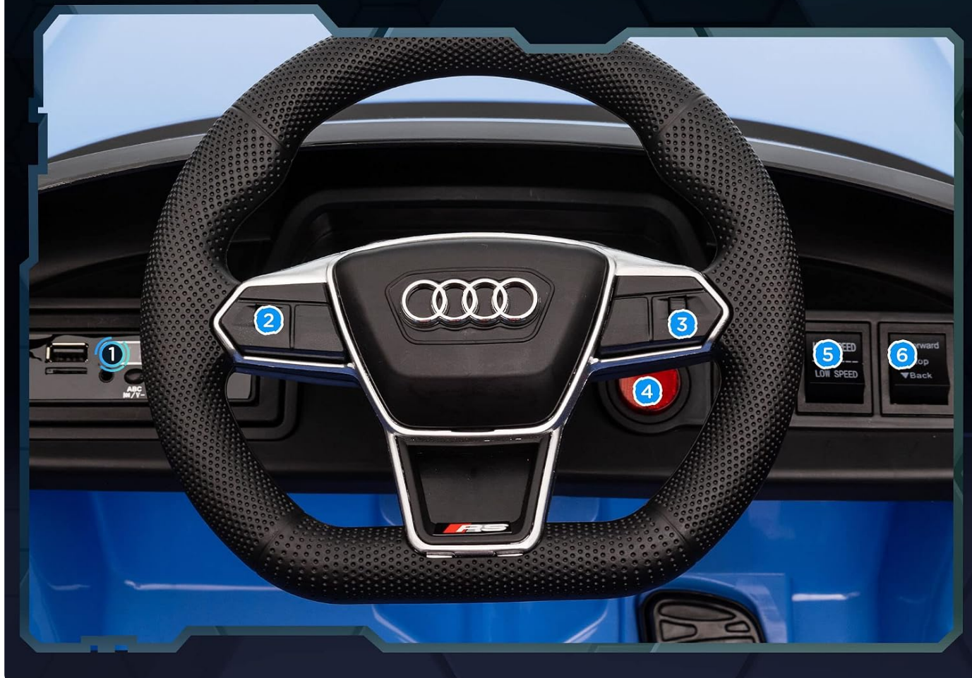
Figure 4: Dashboard controls including MP3 player, horn, music, on-off, speed, and direction switches.
