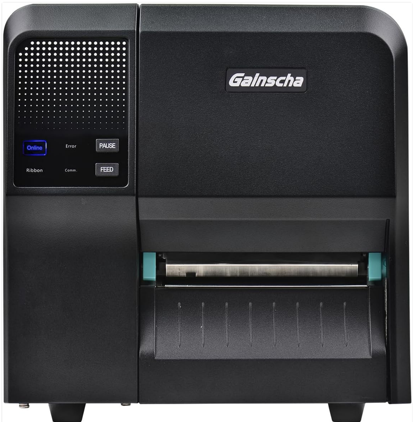
Figure 3.1: Front control panel with Online, Error, Pause, Ribbon, Comm, and Feed indicators/buttons.
