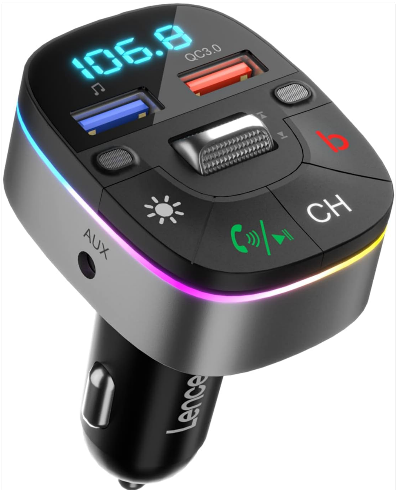
Figure 1: Front view of the LENCENT T75 Bluetooth FM Transmitter, showing the digital display, two USB charging ports (one QC3.0, one standard), an AUX port, and various control buttons including call answer/end, channel selection, and bass boost.
