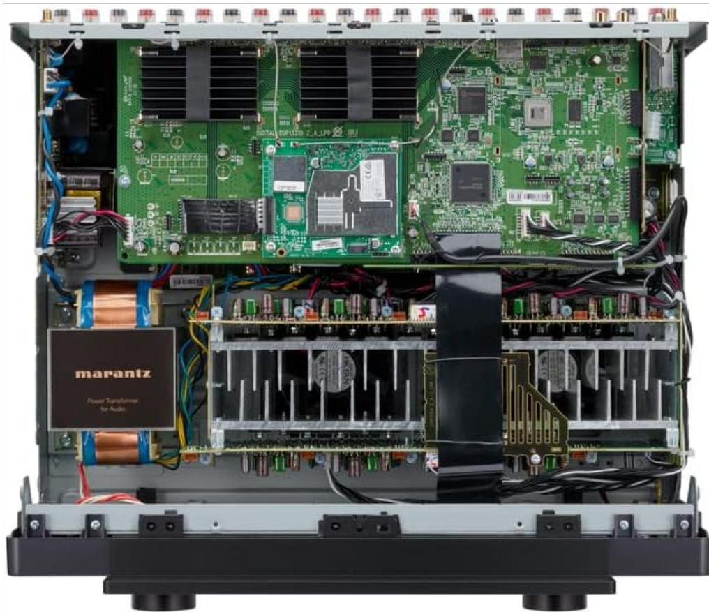
Figure 4: Internal view of the Marantz Cinema 50, highlighting the design for heat dissipation.
