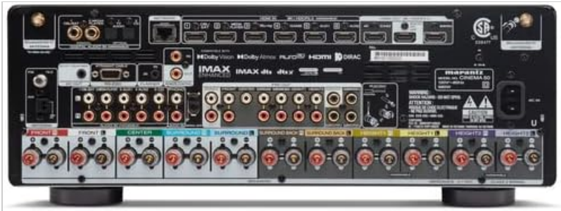
Figure 2: Rear panel connections of the Marantz Cinema 50.
