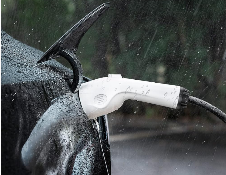
Figure 4: The waterproof IP66 rated control box and connector in an outdoor environment, demonstrating resistance to rain and moisture.
