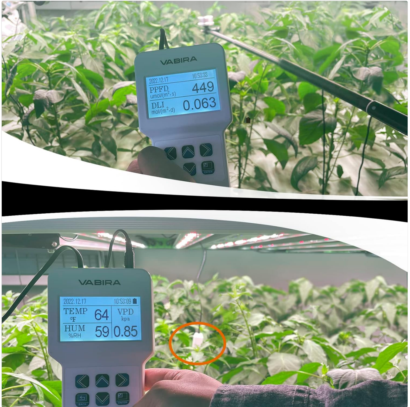
Figure 4: The VBR-200 displaying PPFD and DLI measurements in a plant growing environment.
