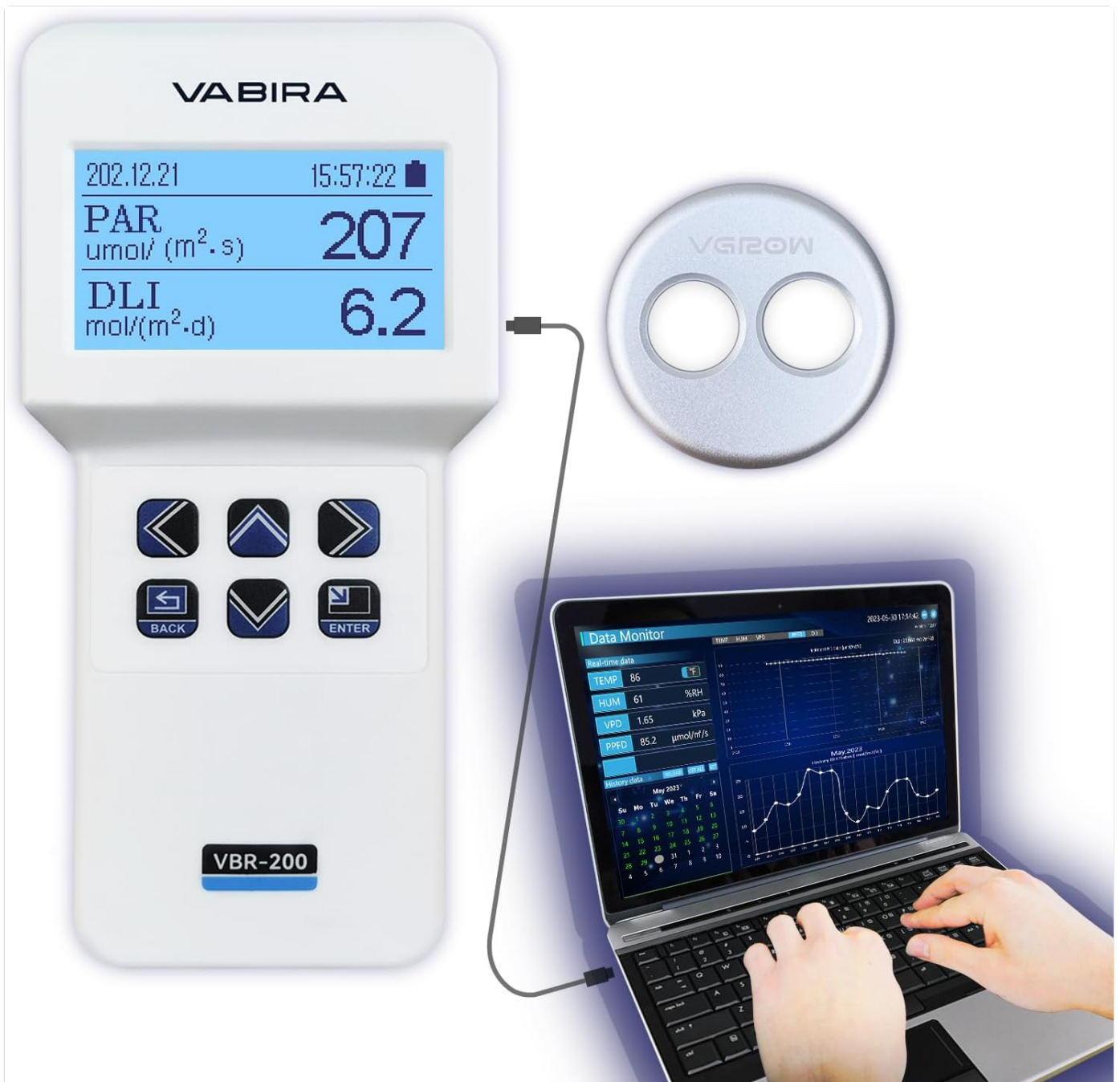
Figure 1: VBR-200 PAR Meter connected to its sensor and a laptop for data monitoring.
