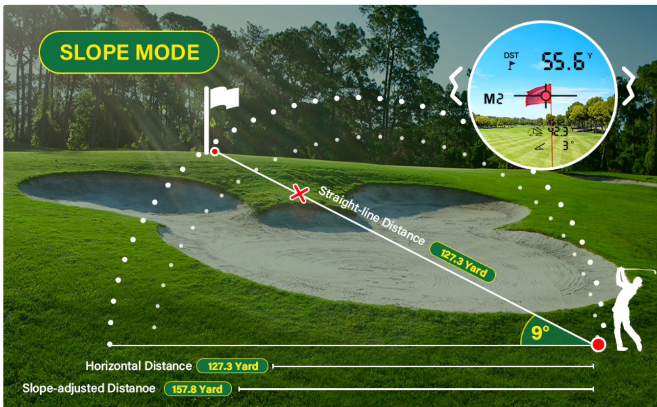
Image: Diagram illustrating the Slope Mode, showing the straight-line distance, horizontal distance, and slope-adjusted distance to a target on an incline.
