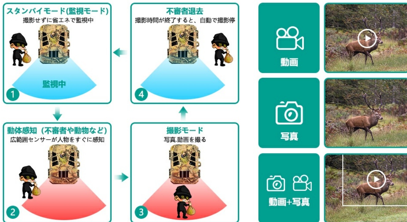
Figure 5.1: PIR Motion Detection Recording Modes
