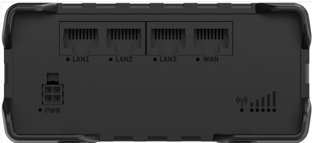
Figure 4: Bottom view of the RUT951, showing the Ethernet ports and power input.
