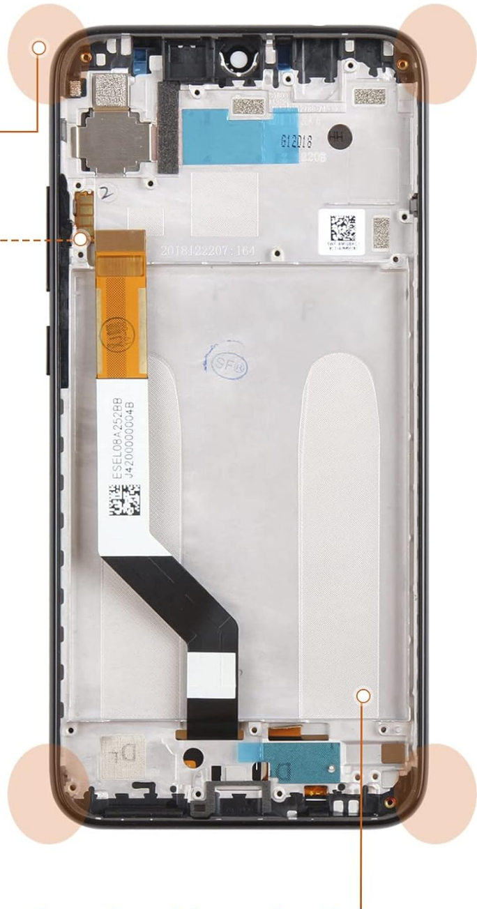
Image 4: Diagram illustrating critical areas to avoid pressure (screen edges, corners, chip) and a warning against folding or pulling the flex cable.
