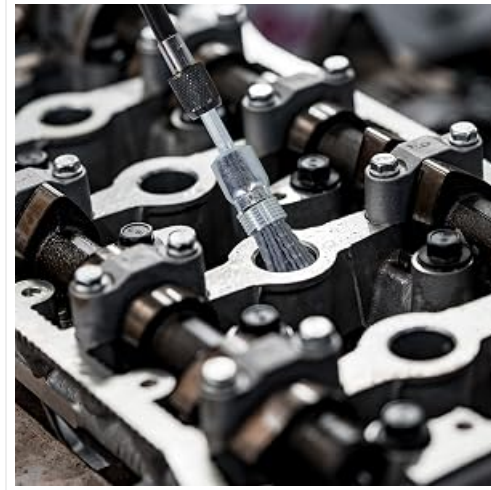
Figure 5: Demonstrating the use of a brush to clean an injector well within an engine block.
