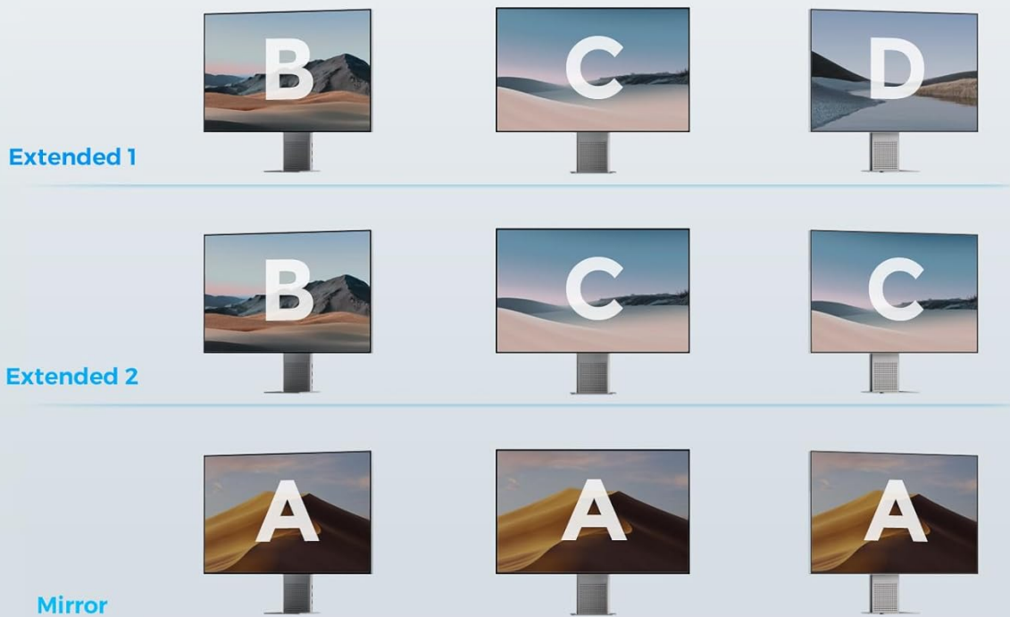
Image: Illustrates various display configurations (extended and mirrored) for Windows and macOS using DisplayLink technology.
