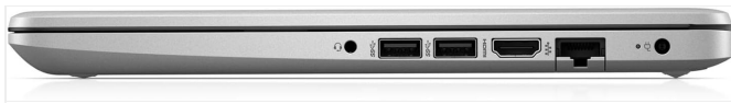
Image: Close-up of the right side of the HP 245 G9 laptop, showing the audio jack, two USB-A ports, an HDMI port, an Ethernet port, and a security lock slot.
