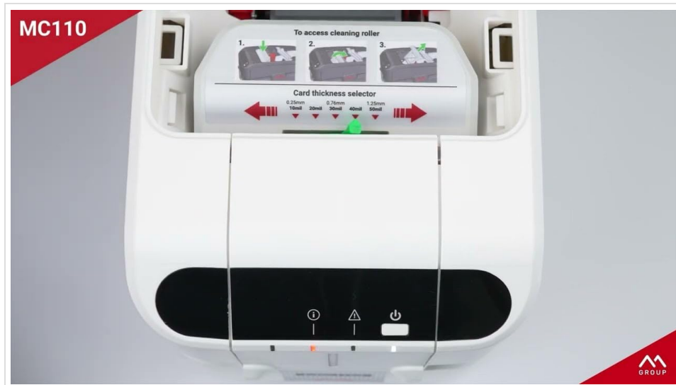
Figure 2: Internal view of the Matica MC110 printer, highlighting the card thickness selector.
