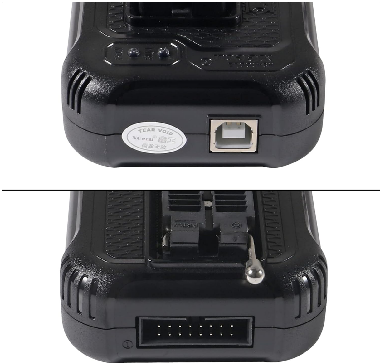
Image: Close-up view of the T48 programmer showing the USB port for connection to a computer and the 16-pin ISP header for in-system programming.
