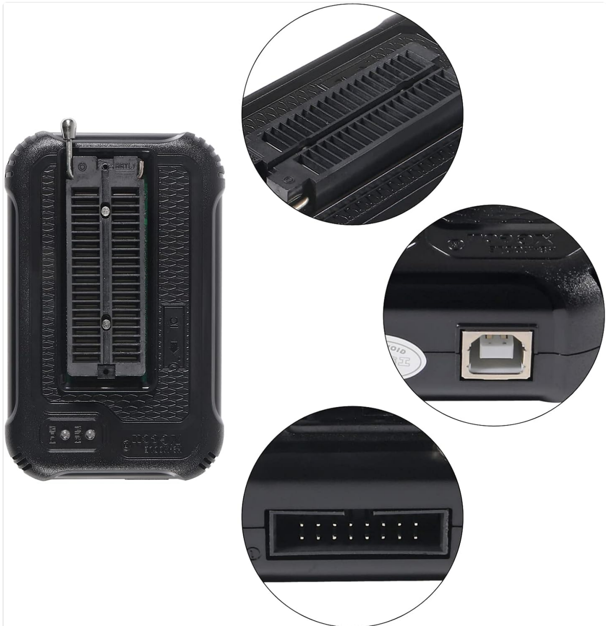
Image: The T48 programmer shown with magnified views of its key interfaces: the ZIF socket for IC insertion, the USB port for computer connection, and the ISP header for in-system programming.
