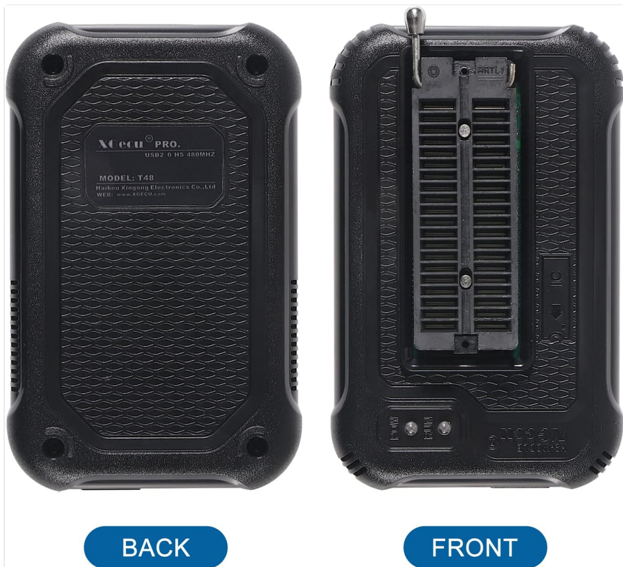
Image: Front and back view of the ACEIRMC T48 TL866-3G Universal Programmer. The front features the ZIF socket, while the back shows product labeling.
