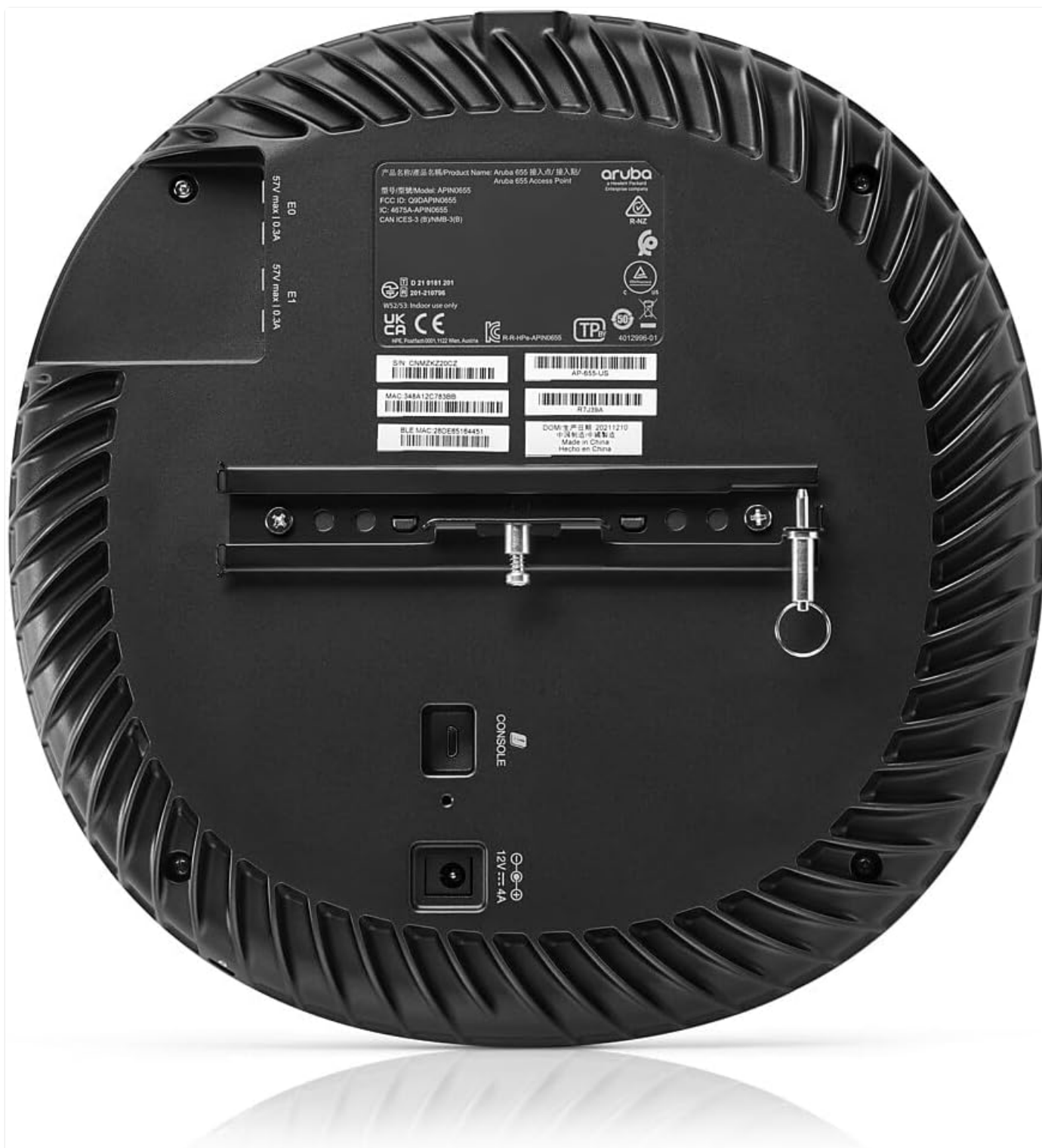
Figure 2.2: Rear view of the HP Aruba AP-655 Wireless Access Point. This view displays the back panel with ventilation grilles, product labels, and various connection ports. A mounting bracket is attached, and ports for console, power (12V === 4A), and two Ethernet ports (E0, E1) are visible, along with regulatory information.
