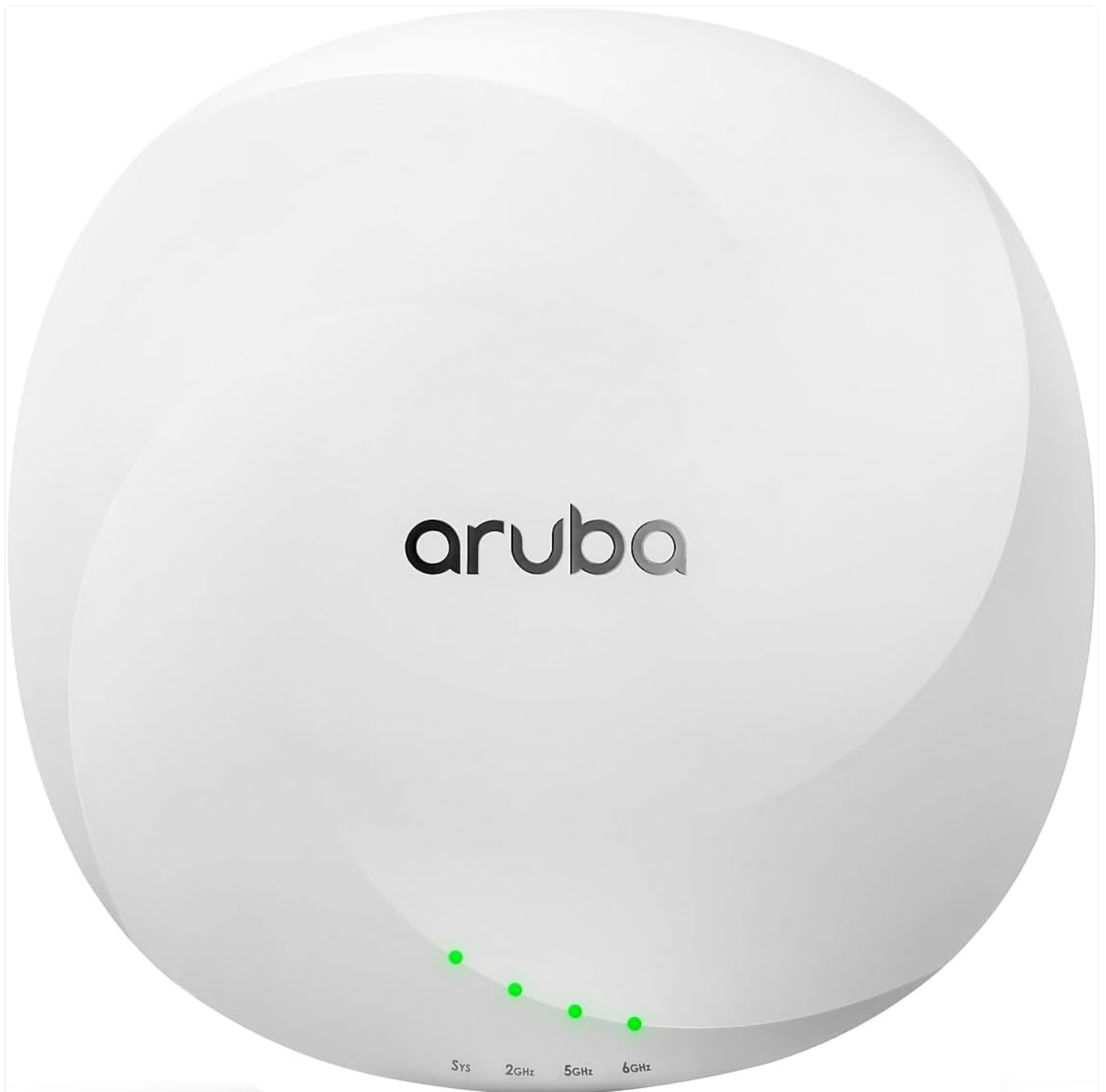
Figure 2.1: Front view of the HP Aruba AP-655 Wireless Access Point. The device is white and circular, featuring the 'aruba' logo prominently on the top surface. Below the logo, four small green LED indicator lights are visible, labeled 'Sys', '2GHz', '5GHz', and '6GHz', indicating system status and band activity.
