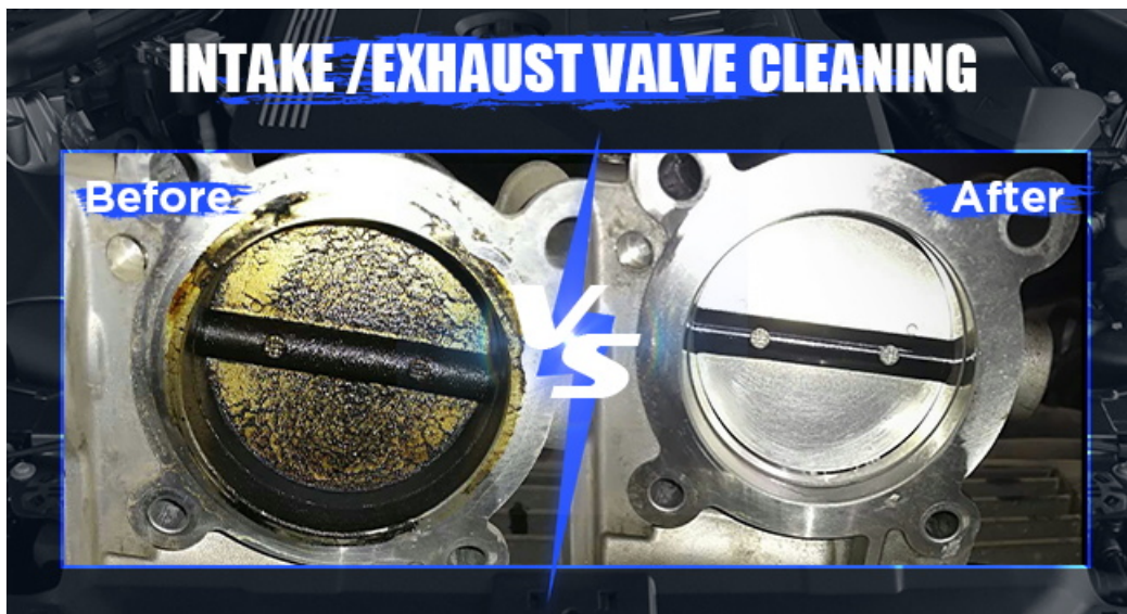
Figure 8: Before and after cleaning of engine intake and exhaust valves.
