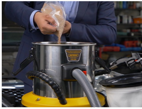
Figure 3: Pouring walnut sand into the machine.
