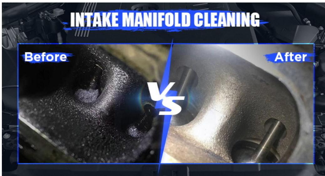
Figure 7: Before and after cleaning of an intake manifold.
