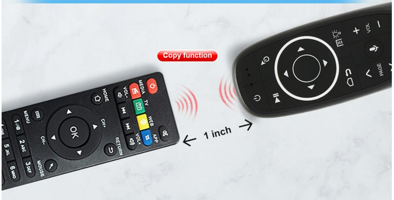
Image: Infrared learning in action, showing the proximity required.
