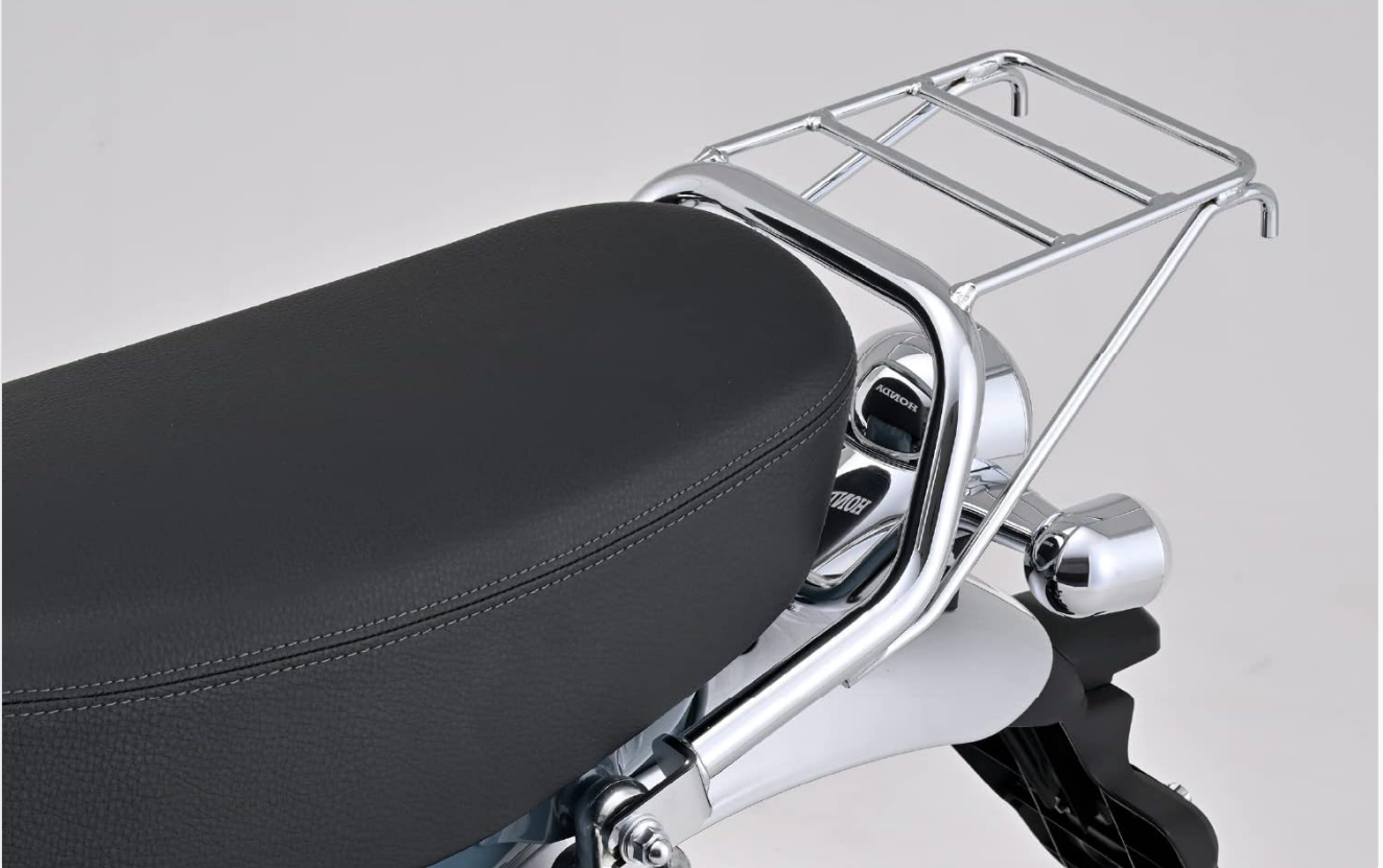
Image 5.2: The carrier is compatible with GIVI universal bases. Please use GIVI boxes 27L or smaller to prevent potential damage to the frame or carrier.
