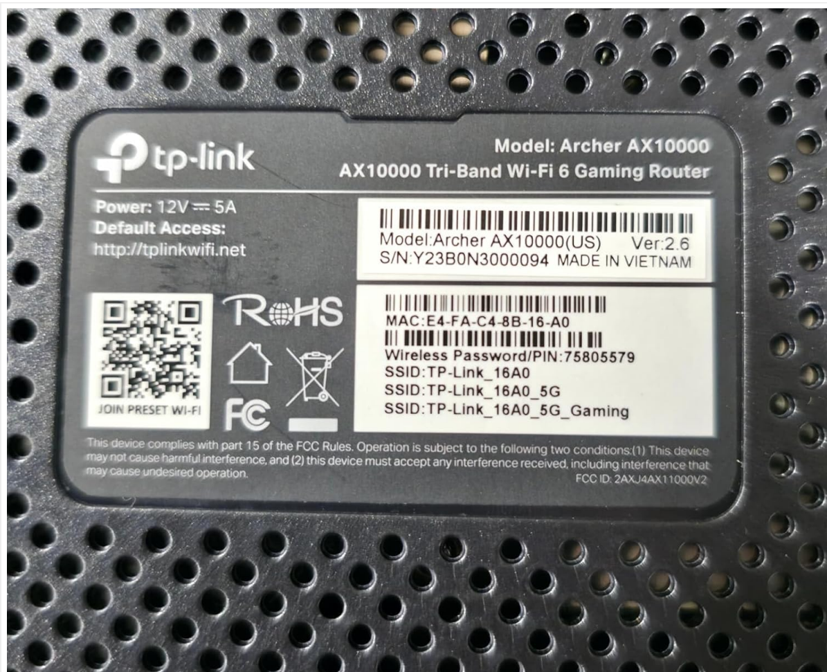
Figure 3: Product label on the bottom of the router, displaying model number, default access information, and wireless password/PIN.
