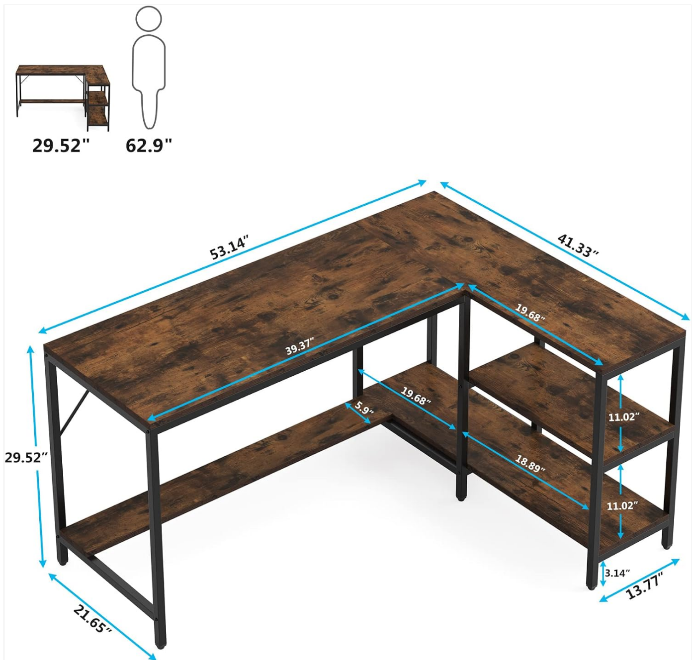
Image: A technical drawing illustrating the full dimensions of the L-shaped desk, including the main desktop lengths (53.14" and 41.33"), height (29.52"), and shelf dimensions, alongside a human silhouette for scale.
