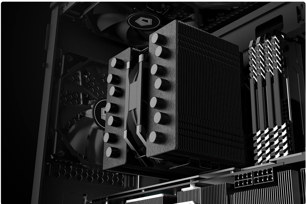
Figure 7: The SE-207-XT Slim CPU Cooler installed in a PC case, viewed from the side, showing its compact height and RAM compatibility.
