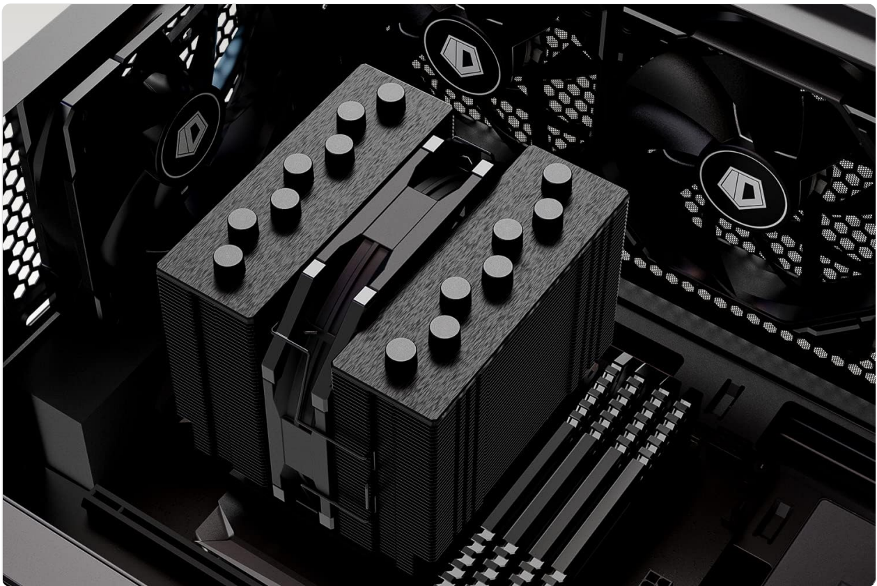
Figure 6: The SE-207-XT Slim CPU Cooler installed within a PC case, viewed from above, demonstrating its fit and clearance.
