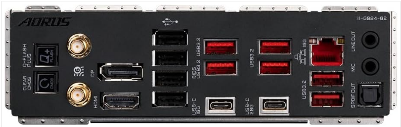
Image 4.3: Detailed view of the rear I/O panel on the Gigabyte X670E AORUS XTREME Motherboard. This panel includes multiple USB ports (USB 3.2 Gen 2x2 Type-C, USB 3.2 Gen 2 Type-A), a 10G LAN port, Wi-Fi 6E antenna connectors, audio jacks (including S/PDIF Out), HDMI, DisplayPort, and Q-Flash Plus/Clear CMOS buttons.
