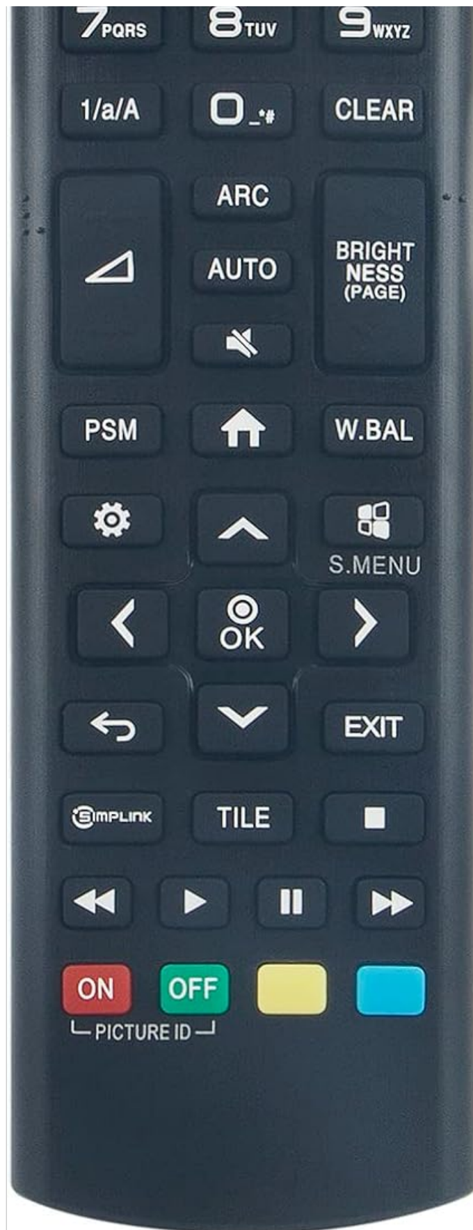
Figure 2.1: Front view of the remote control. This image displays the layout of all buttons, including power, number pad, channel, volume, navigation, and media controls.
