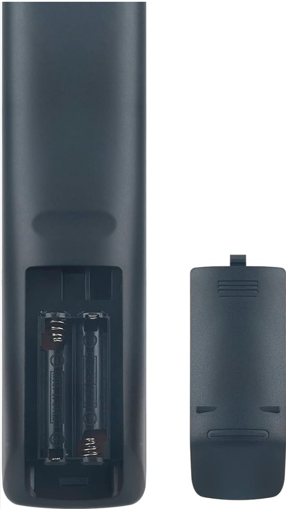
Image: Rear view of the remote control with the battery cover removed, illustrating the correct placement for two AAA
