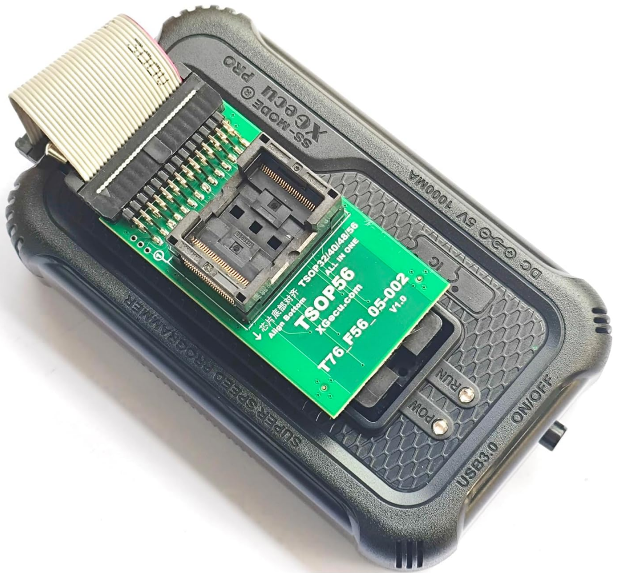
Figure 7: T76 Programmer with a TSOP56 adapter connected.
