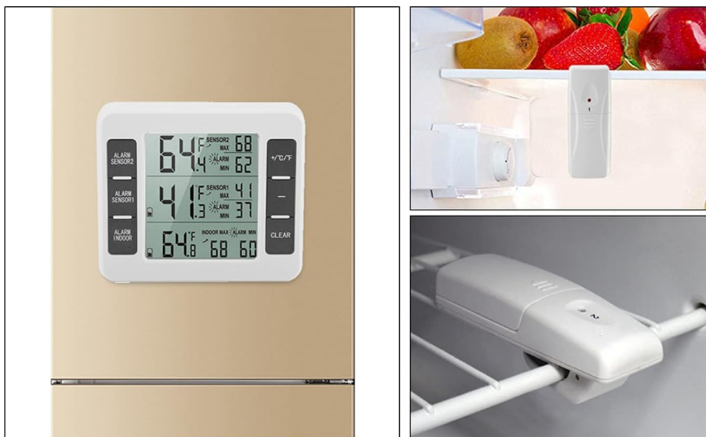
Image 4.2: Example of remote sensors placed inside a refrigerator and freezer compartment, demonstrating their compact size and clip attachment.
