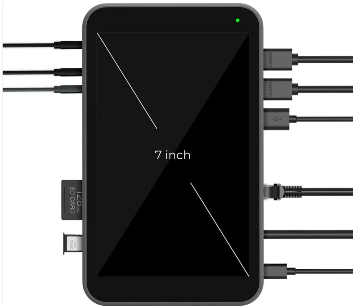
Figure 3.3: The YOLOLIV Instream connected to various inputs and outputs, including HDMI cameras, USB devices, and network cables, demonstrating its connectivity options.
